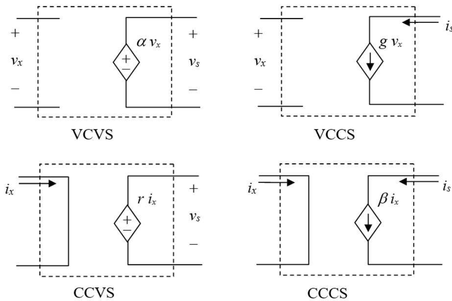
VCVS: Voltage-Controlled Voltage Source
